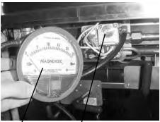
MANOMETER REGULATOR Step 1a ADJUSTING SCREW
