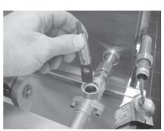
c. Remove the core-disc assembly, core spring retainer, and the core spring.
