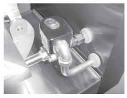
1. Remove Tru-Arc retaining clip on top of the coil housing.
